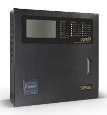
WISE Control Panel is an addressable fire alarm control panel with the capability to address and manage all events of connected devices. The possibility to integrate ten loop expanders into a single system makes the panel suitable for use in small to large buildings and installations. The panel has a modular structure which further helps in designing a wide range of projects.
