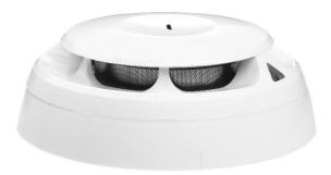
S6-CMD-200 is a multi-sensor detector that combines a smoke detector and a fixedtemperature heat detector. It detects smoke in the environment and measures ambient temperature with its temperature-sensitive sensor. It becomes active in temperatures above 62 °C and will trigger a fire alarm when its smoke sensor detects the presence of smoke in the environment.
