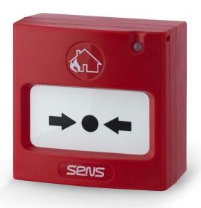
The S6-ACP-300 is an addressable resettable fire alarm call point, one of the non-automatic components of fire alarm systems. It can be reset using the supplied key and is equipped with a front LED.
