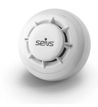
S2-CMD-200 is a multi-sensor detector that combines a smoke detector and a fixed-temperature heat detector. It detects smoke in the environment and measures ambient temperature with its temperature-sensitive sensor. It becomes active in temperatures above 70 °C and will trigger a fire alarm when its smoke sensor detects the presence of smoke in the environment.
