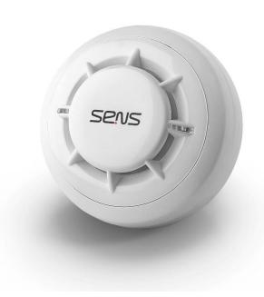
S2-ARD-300 is the addressable rate-of-rise heat detector, designed based on the measurement of temperature and its rate of growth. It responds to sudden temperature increases as well as temperature rising above a certain level. The detector's performance is regulated according to standards and activates at a temperature growth rate of 8 degrees Celsius per minute. It is suitable for locations where smoke-producing materials are present and environments where fire rapidly escalates.
