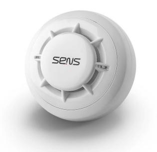
S2-AHD-300 is addressable Fixed Heat Detector, using Temperature a temperature-sensitive sensor. When the temperature in the surrounding area reaches over 70°C, it reports a fire alarm to the central panel. This detector is suitable for locations where smoke-producing substances exist under normal conditions.
