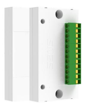
Addressable output modules with loop-powered technology are installed in a loop along with other connected components to the control center, such as detectors, push buttons, sounders, etc., without requiring an external power supply.
