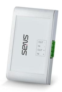
I1-AIS-300 is an isolator module that is used to isolate the circuit in the event of a short circuit in the loops of the addressable control center. If a short circuit occurs in a part of the wiring route that is isolated by this module, the connection of that part will be separated from the other parts of the circuit. So, the other elements will continue to their normal function without any disturbance.
